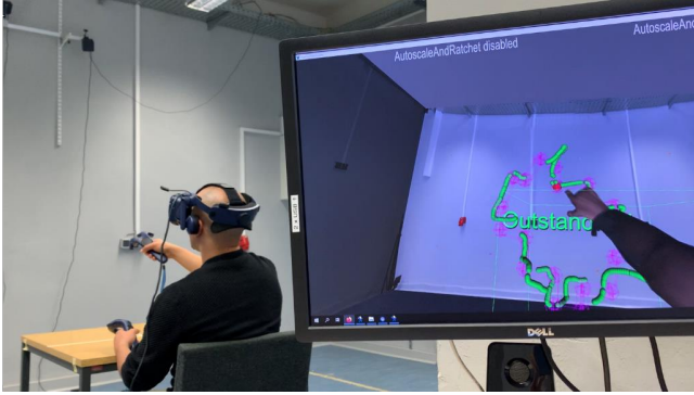
Figure 1: Experimental setup. The screen in the foreground shows the view of the participant’s HMD. The green line represents the participant’s drawn trace inside the magenta 3D figure.
