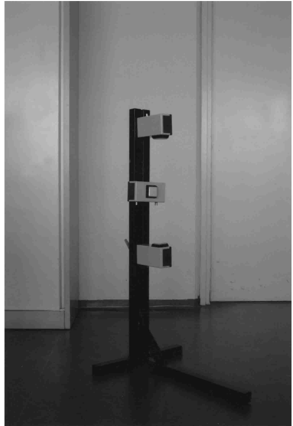
Figure 1. The experimental setup used in Experiments 1, 2, and 3. Three one-button boxes were fixed on a stand. Both response buttons were positioned perpendicularly above and below the home button. Participants were instructed to push the upper or lower button in response to a stimulus, and they consequently flexed or extended their arm, respectively.
